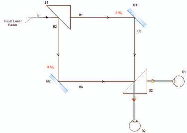
Fig. 2: The Mach-Zehnder interferometer in the classical mode
