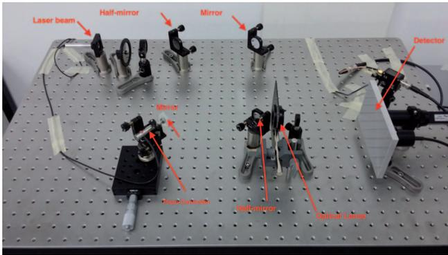
Fig. 5: Preliminary physical setup of the Mach-Zehnder Interferometer
