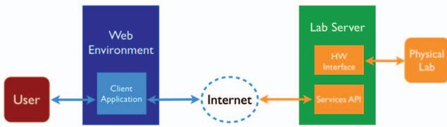
Fig. 1: The Smart Device architecture for remote labs
