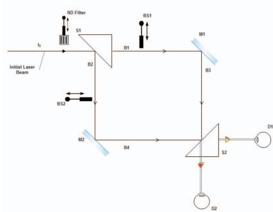
Fig. 4: The Mach-Zehnder interferometer in the quantum mode
