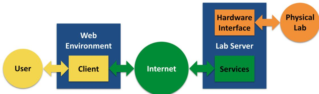
**Figure 1. The remote lab architecture (taken from D4.1)**
