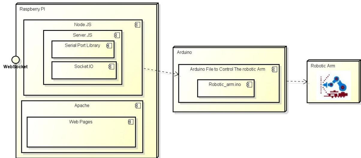
**Figure 8. Robotic Arm deployment architecture**
