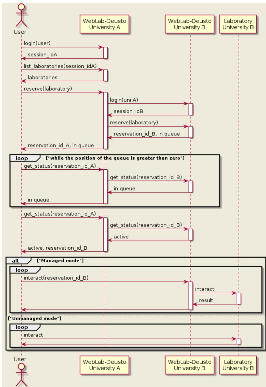
**Figure 14: Federation algorithm in WebLab-Deusto**
