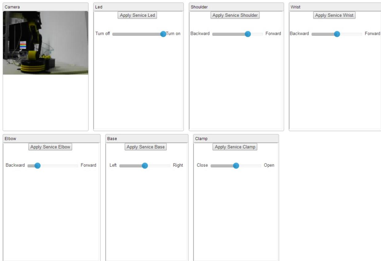
**Figure 9. The simple client app integrated in Graasp (video and actuators controls)**
