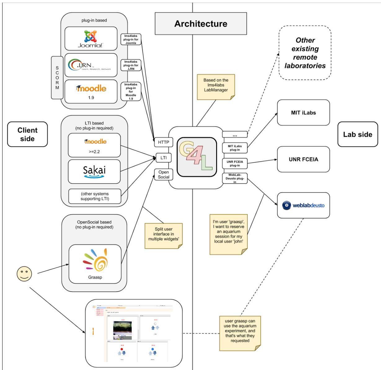
**Figure 11: Gateway4Labs overall architecture**
