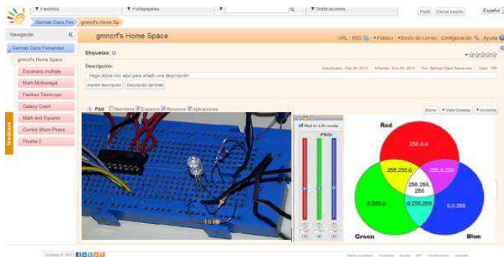
Figure 4. The RGB LED lab integrated in an inquiry learning space. The various Web apps connect to the specified services (video stream, actuators).
