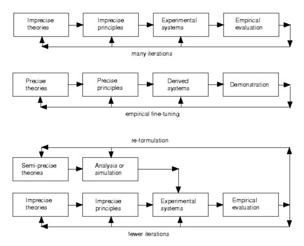
Figure 3. The ITS design process
