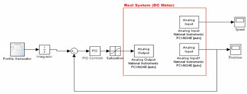
(b). closed loop with PID controller.
