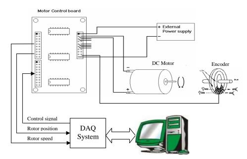
Fig. 5: Experiment setup for DC motor control
