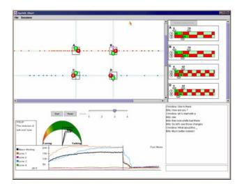
Figure 3: COTRAS (Collaborative Traffic Simulator). The group mirror is the red-green meter with 3 arrows, one for each user and one for the group. (Jermann, 2004)
