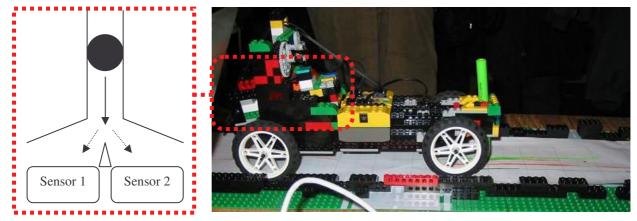
**Fig. 3:** On the right, the Drunk Bot is free to move on a lane, leaving a coloured trace thanks to a pen. The Roller device consists of a transparent component of the robot which is explained by the left picture. A marble slides down and hits a pin, then it may go left or right (randomly), thus hitting sensor 1 or sensor 2. The Drunk Bot moves a step backward or forward according to the hit sensor.
