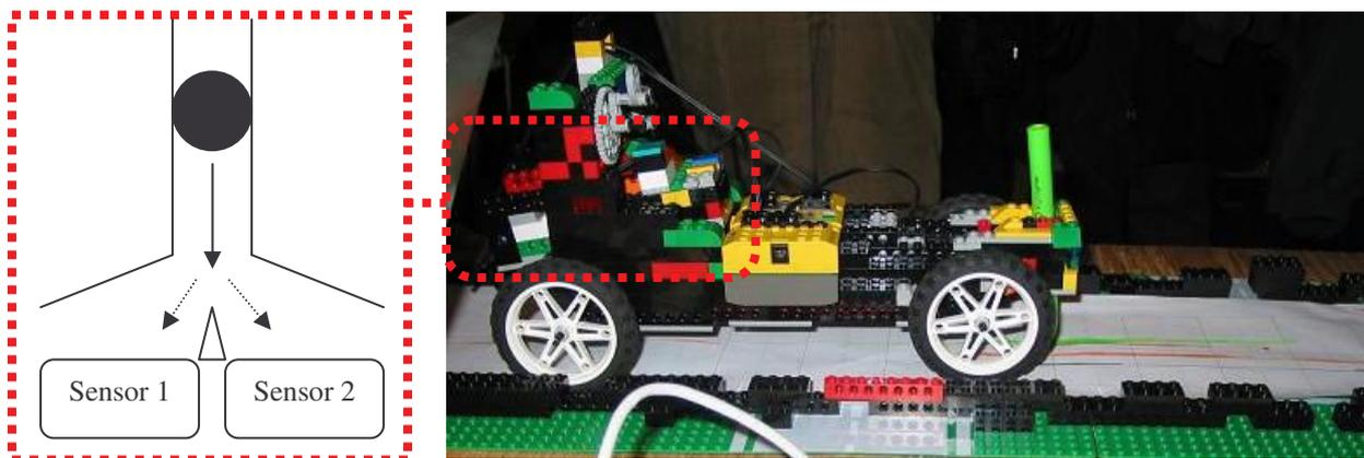
**Fig. 3:** On the right, the Drunk Bot is free to move on a lane, leaving a coloured trace thanks to a pen. The Roller device consists of a transparent component of the robot which is explained by the left picture. A marble slides down and hits a pin, then it may go left or right (randomly), thus hitting sensor 1 or sensor 2. The Drunk Bot moves a step backward or forward according to the hit sensor.
