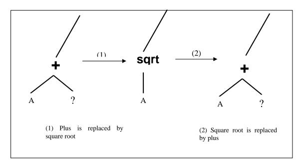
Figure 24. Modification of an internal node in controlled mode when a change of arity is possible by deletion or insertion of empty children.
