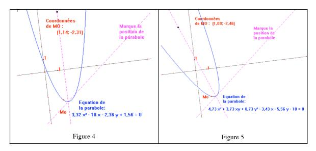
Different positions of the parabola in Cabri
