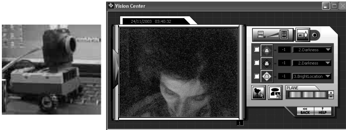
Figure 10.17. A simple robot for gathering visual data using digital camera, and the screen to process captured image
