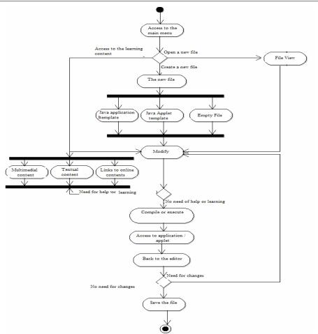
FIGURE 2. The conceptual and functional architecture design of the JAVA learning environment
