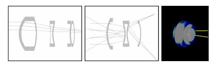
FIGURE 10. A zeites optical system reconstructed in the optics module, a system with mirror surfaces and a 3D view of an optical system
