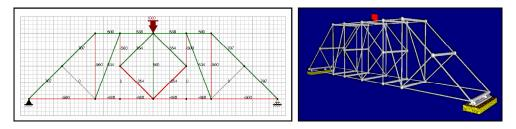
FIGURE 11. A bridge and its 3D model built with truss analysis module
